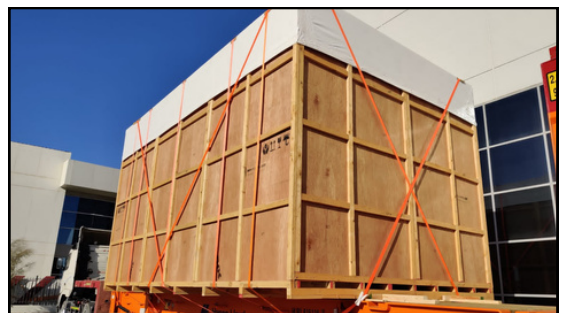
Safe Transport Using 40 FR Container with Professional Lashing Solutions
