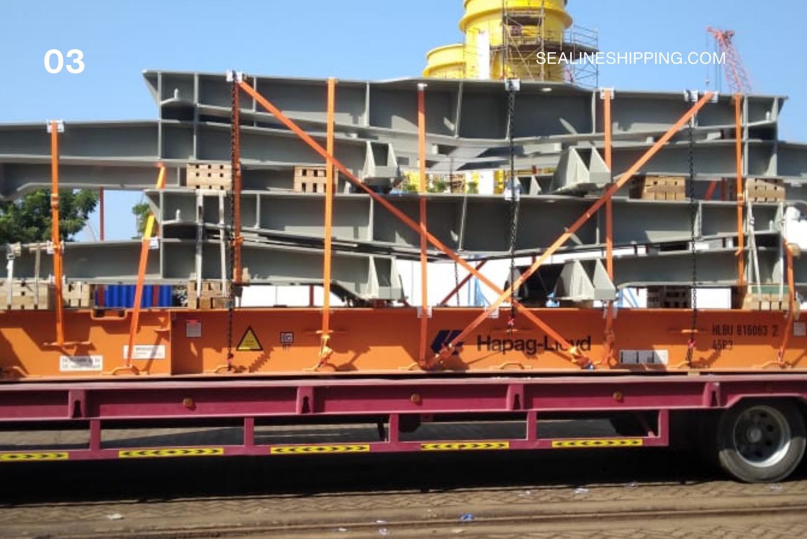
Precision Handling of Steel Structure Columns via 40 FT FR Container
